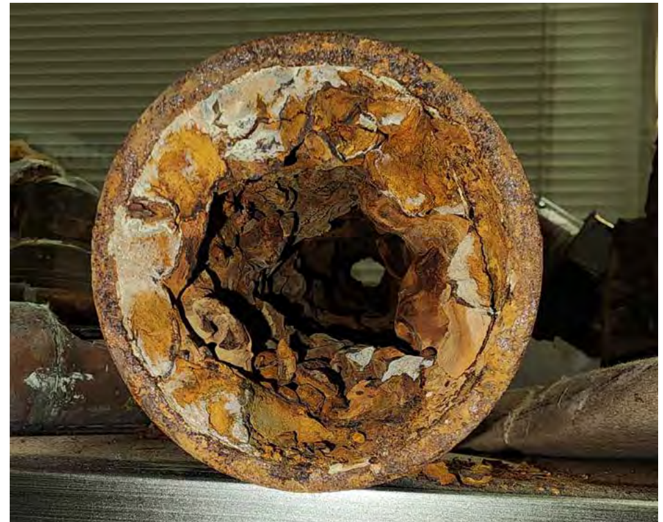
Example of pipe corrosion and buildup over time
